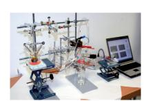
Forever blowing bubbles: Hydrogen is generated from formic acid amine adducts at room temperature used directly in fuel cells (see picture for apparatus). Ruthenium phosphine systems act as catalysts in this transformation.
